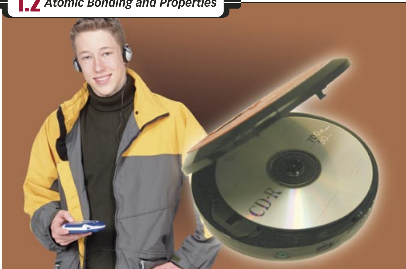
Figure A1.3: Music CDs are made from a type of plastic called polycarbonate.
