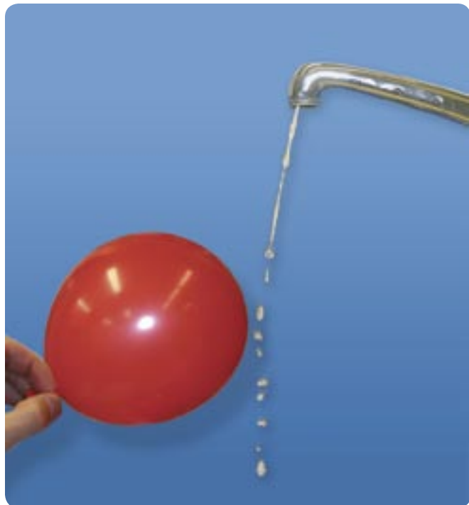
Figure A1.10: A balloon that is statically charged will bend a stream of water without touching it.
