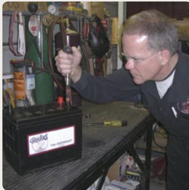
Figure A1.23: A battery technician checks the concentration of sulfuric acid.
