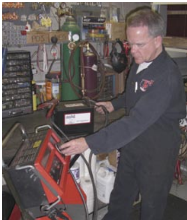
Figure A1.24: The voltage output of an automotive battery is checked.
