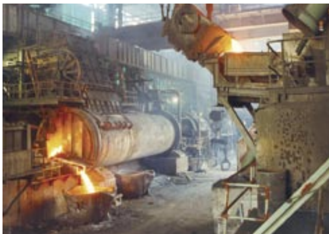
Figure A2.8: Blister copper is poured after being removed from a furnace.
