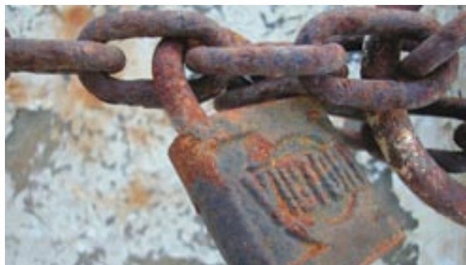
Figure A2.17: Iron readily corrodes if it isn't sufficiently protected from the environment.
