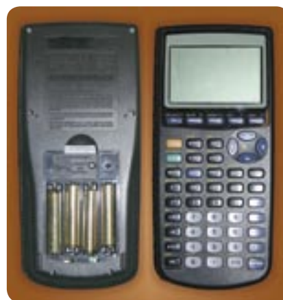
Figure A1.21: This calculator is powered by a battery of four voltaic cells.
