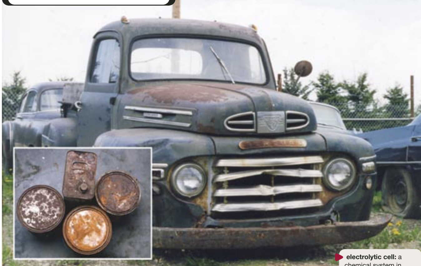
Figure A2.26: Iron is an easy victim for corrosion if left unprotected.
