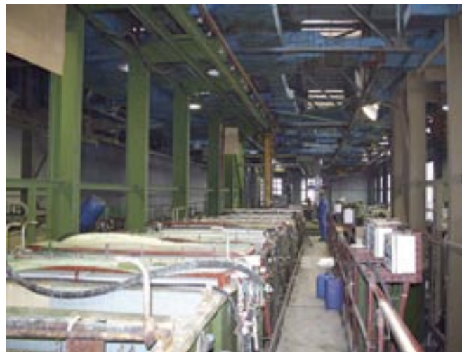
Figure A2.27: Large-scale industrial electroplating facilities use banks of electrolytic cells to produce metal coatings.
