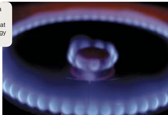
Figure A3.19: When the ratio of oxygen to fuel is right, hydrocarbons burn with a blue flame.
