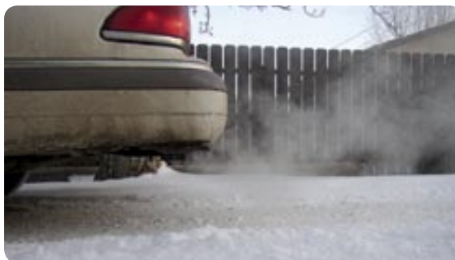
Figure A3.20: It is the condensed water vapour in the exhaust from a vehicle that makes it visible.
